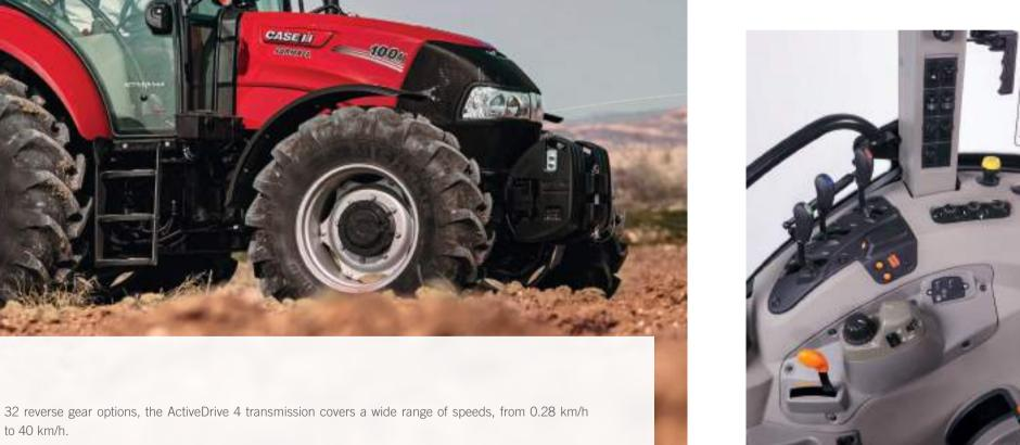
Auxiliary equipment such as the electro-hydraulic power shuttle, power shuttle sensitivity settings, automatic 4 WD, automatic differential lock, and buttons for easy gear shifting, ensures that maintaining high levels of operating efficiency is never at the expense of comfort, which remains paramount in the equipment design.
