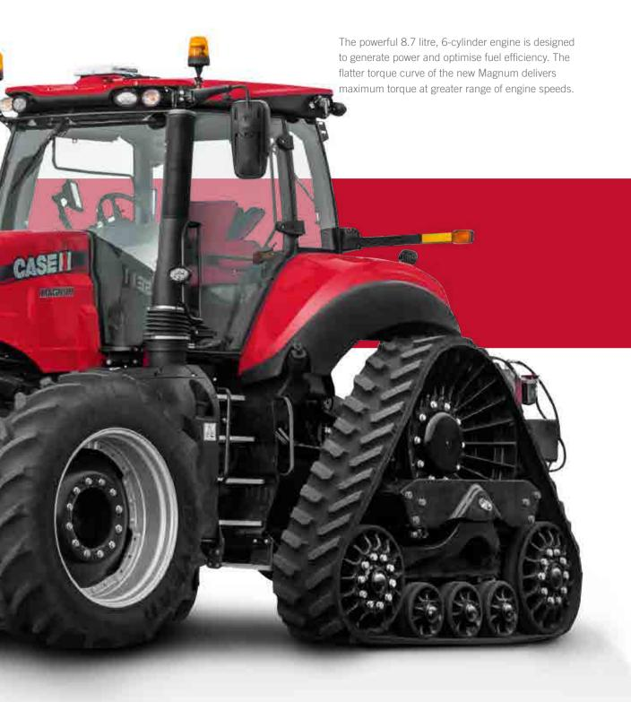
You can choose the proven Full Powershift Transmission with Automatic Productivity Management (APM) that automatically reduces engine speed to match power requirements. Or you can opt for the Continuously Variable Transmission that makes the Magnum CVT the perfect all-rounder on the road and in the field, with the CVT speed range from 0 to 50 kph.
